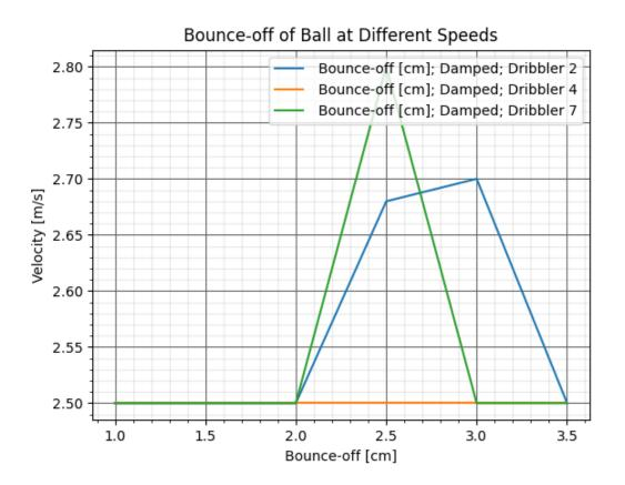
Robot nr: 15 (barely any damping) Dribbler: 2/7 Robot stationary Gear ratio: small(motor) to big(dribbler)
