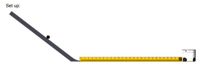
The ball will be dropped from different heights in order to test the damping behaviour for various ball velocities. The approximate velocities that have been used during the test are 1.0 m/s, 1.5 m/s, 2.0 m/s, 2.5 m/s, 3.0 m/s, 3.5 m/s. The maximum allowed speed for the ball during a game
