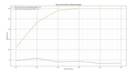
Robot nr: prototype new FA PETG flexure Dribbler: off Robot stationary
